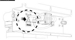
The Flow Restrictor is installed inside of the red tube at the bent end connected to the Drain port on the back of the RO module. DO NOT REMOVE THE FLOW RESTRICTOR OR CUT THE RED TUBING AS IT WILL DAMAGE THE FLOW RESTRICTOR.
